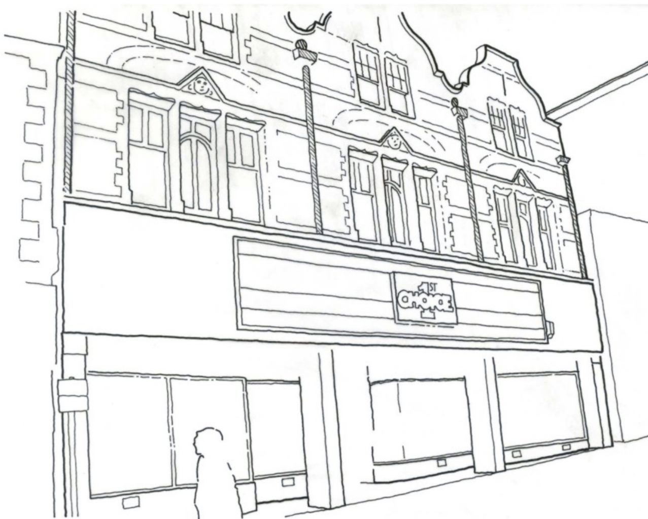
Figure 2. This excessively large fascia sign overpowers the building and street scene
