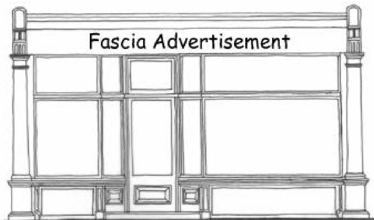
Figure 1. Traditional Signage usually takes the form of a hand painted fascia sign
