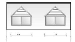
On less prominent elevations the width of any dormer window should not exceed two thirds of length of the base of the roof plane to which it is attached.
