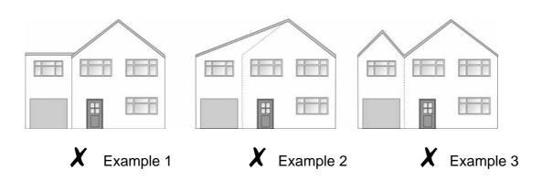
3.5 The flat roof in example 1 is an ugly and inferior form of construction, and is visually and physically at odds with the pitched roof. The unequal roof pitch created by the extension in example 2 unbalances the whole elevation, whilst the proportions and roof pitch of the extension shown in the third are incompatible with the original.
