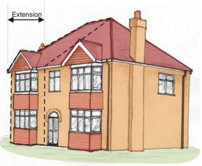
Left : With care, good design and appropriate use of materials, even older properties can be extended in a sympathetic manner. Note how the window design and positioning reflect those of the existing building.
