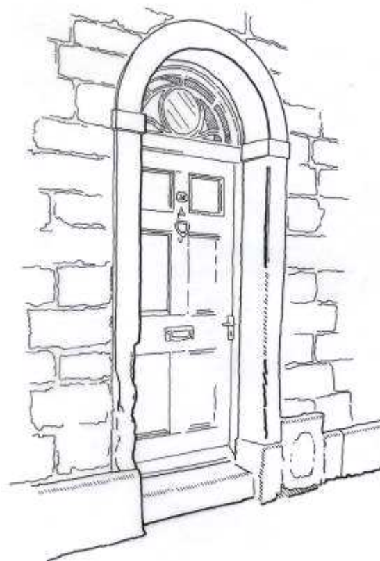
A round headed door case with imposts, a cast iron fanlight and a blocked boot scraper, containing a six panel door.
