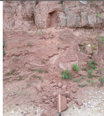
Photograph 6a and 6b: Small Ravel Failure Behind Unit 6 / 7 Boundary. (Images taken 30/04/2020).
